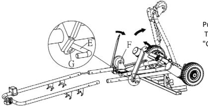
Pull up the wheel frame "F" as shown. Twist each support arm to lock groove "G" into position on the cross bar "E".
