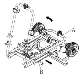
Insert the support arm "B" and "C" to each shaft of the frame in the direction of the arrow.
