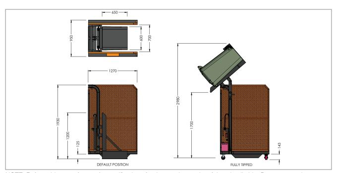
NOTE: Refer to bin manufacturer's specifications for the rated capacity of the wheelie bin. Do not exceed wheelie bin capacity without the manufacturers approval. The typical capacity for a 240L bin is approx. 100kg.
