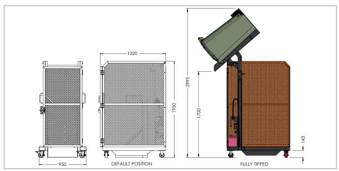
NOTE: Refer to bin manufacturer's specifications for the rated capacity of the wheelie bin. Do not exceed wheelie bin capacity without the manufacturers approval. The typical capacity for a 240L bin is approx. 100kg.
