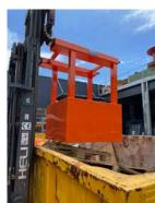
MFCA110 Bin Compactor is designed to safely and effortlessly compact bulky waste products such as cardboard and plastic with approx. 1T weight.
