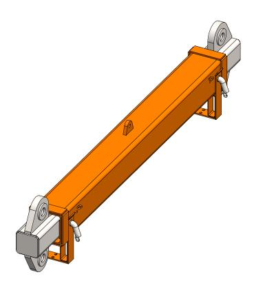
The type LCEH2439 Spreader Beam (Heavy) is a heavy duty crane spreader beam. The spreader beam is designed to suit over-head cranes and is supplied with 2 retaining brackets for storage. Loads should be end lifted using two end lifting lugs along with 2 leg chain sling.
