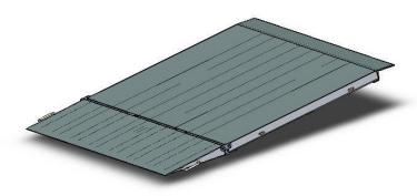
The type MCRN8 Container Ramp is designed for bridging into standard containers from ground level. The self-levelling lip allows for full load capacity when on slightly uneven ground.
