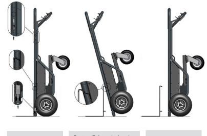
Flat Plate Attached and Locked.
