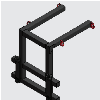
Lifting Frame with fork carrier brackets fitted allows mounting to a fork carriage
