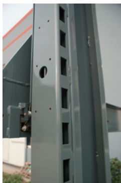
- Dynamic locking device With 6 locking tabs
